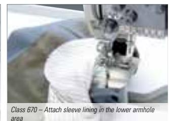
*Class 670 – Attach sleeve lining in the lower armhole area*
