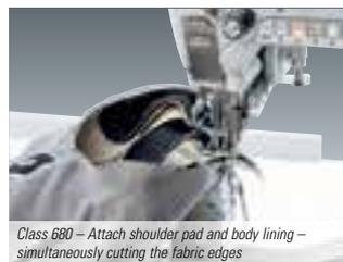
*Class 680 – Attach shoulder pad and body lining – simultaneously cutting the fabric edges*
