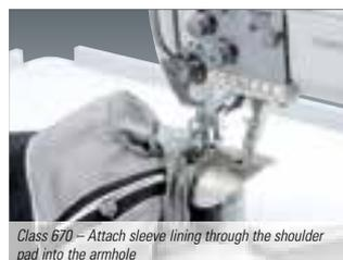
*Class 670 – Attach sleeve lining through the shoulder pad into the armhole*
