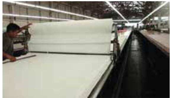
*In case of automatic spreading, the number of workers required to handle the fabric reduces to one*
