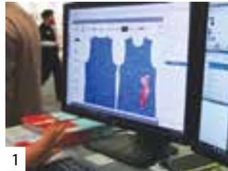
1 *Assyst Vidya 3D-simulation software creates virtual design of the garment*
